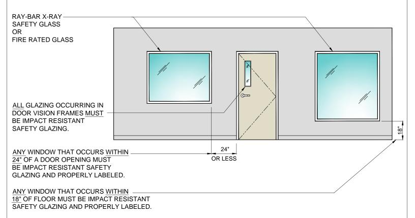
RAY-BAR X-RAY SAFETY GLASS OR FIRE RATED GLASS IS PERMANENTLY LABELED AS MEETING ANSI Z97.1 AND CPSC 16 CFR PART 1201 CAT 2 AS REQUIRED BY IBC 2406 FOR IMPACT RESISTANCE.
